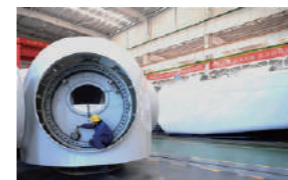
Wind-Driven Generator Assembly
