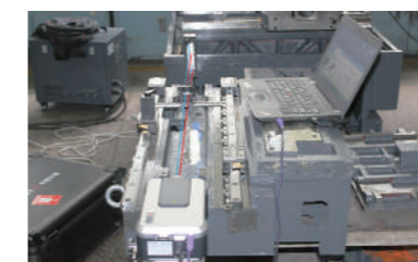
Parallelism meas. of two guide rails
