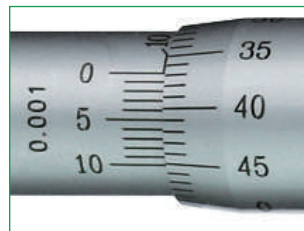
Spindel 0,5 mm - Ablesung 0,001 mm Thread pitch 0.5 mm - Reading 0.001 mm
